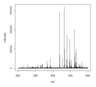
This figure shows one of the mass-spectra (m/z signals). This spectrum corresponds to measurement number 601, which is the measurement done at 3440.3 seconds.
