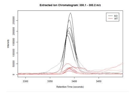
Figure. The extracted ion chromatogram for the mass-slice 300.1-300.2. You see the intensity values for 6 WT and 6 KO samples. The intensities between these two groups are clearly different. Notice that the alignment of the samples was not perfect. Also notice that one of the WT samples does not have a very well defined peak. The reason for this is unclear at this stage but could be investigated.
