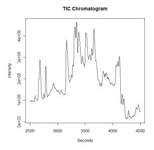
The TIC (total ion current chromatogram). This figure shows the chromatogram' (i.e., the signal in time). The y-axis shows the total 'ion current', which is a summation of all mass-peaks at every time point.
