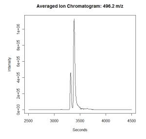
This figure shows the averaged ion chromatogram but because a specific mass was chosen (and not range of masses), it shows how the signal of this specific mass (496.2) varies over time. In other words the compound with this mass elutes from the column after about 3300 seconds.
